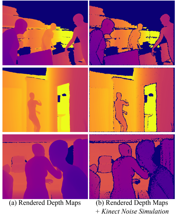
Figure 2: Kinect depth sensor noise simulation. (a) Using the described rendering pipeline, depth maps are rendered from scenes populated with synthetic humans, (b) simulated Kinect depth sensor noise is applied to the rendered depth maps.
